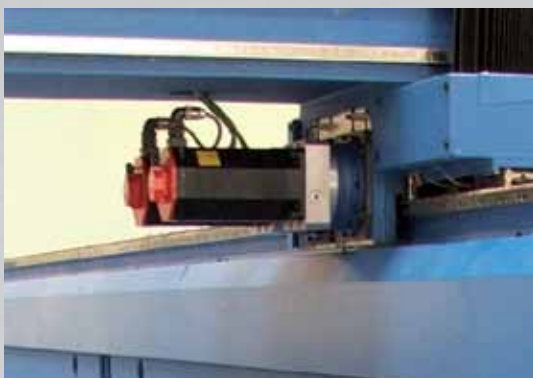
Kinematics with double driving motors on linear axes: backlash recovery, higher rigidity, fast movements
